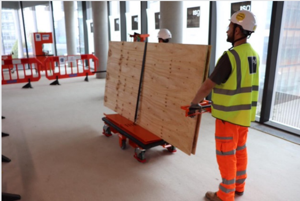
Board trolley with auto-lock break and restraining mechanism
